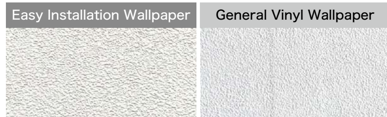
The wallpaper is installed over a substrate with tape applied to simulate unevenness
