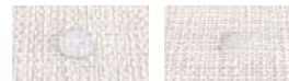
Water Repellent Coating: Water is repelled. General Vinyl Wallpaper: Water droplets spread.
